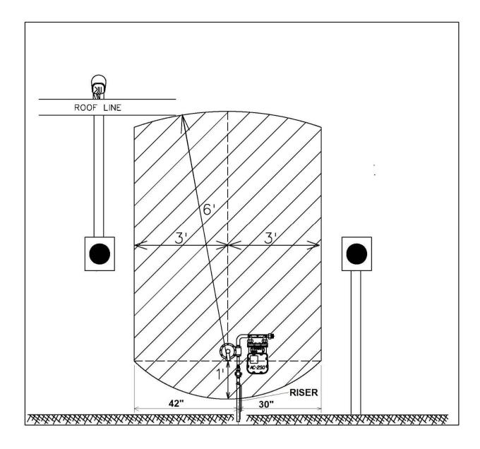
It is recommended that the gas meter be set a minimum of three (3) feet from the electric meter.
