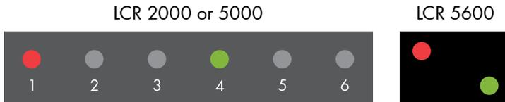
When the LCR 2000 or LCR 5000 is controlling the compressor, LEDs 1, 4 and 5 will be lit on older models. On newer models, only LEDs 1 and 4 will be lit. At all times, disregard LED 5; its status is not relevant to the operation of the LCR. When the LCR 5600 is controlling the compressor, a red LED on the left side and a green LED below and to the right will be lit.
